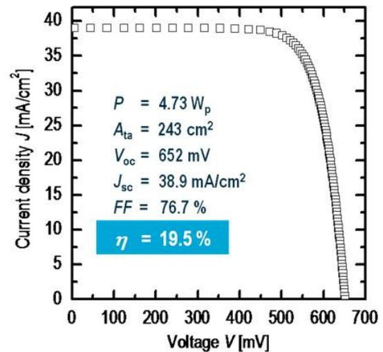
**Figure 5:** *J-V*-curve and parameters of our World Record multi-crystalline large area Q.ANTUM cell. The data were independently confirmed by Fraunhofer ISE CalLab.
