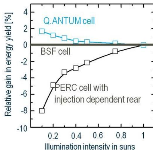
**Figure 8:** Measured and normalized (to 1 sun) energy conversion efficiencies displayed as a relative gain compared to the BSF cell. Our Q.ANTUM technology shows an improved performance at low light intensities.
