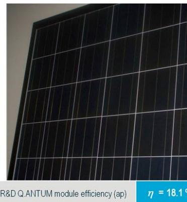
**Figure 6:** Picture of our independently confirmed World Record multi-crystalline R&D Q.ANTUM module.
