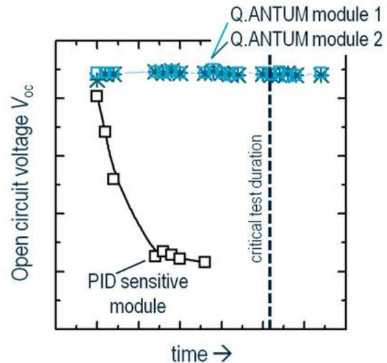
**Figure 10:** Results of a PID test (-600V, wet surface, 25 °C) of two Q.ANTUM modules and one module susceptible to PID. Q.ANTUM includes the Q-Cells anti PID technology and thus shows no degradation effect.
