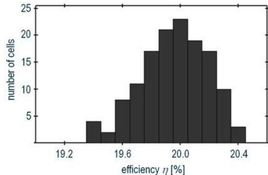
**Figure 3:** Histogram of a R&D run consisting of ~ 130 mono-crystalline Cz Si Q.ANTUM solar cells. We reach a median cell efficiency of 20 % with top efficiencies of up to 20.4 %.
