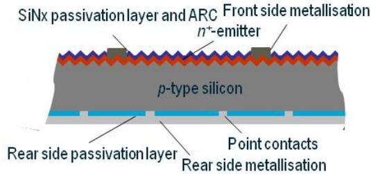
**Figure 1:** Schematic cross-section of the Q.ANTUM solar cell design with passivated rear (not to scale).
