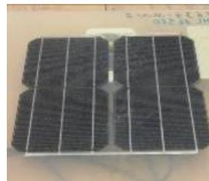
**Figure 8:** Photograph of exemplary mini-module after 1000 hours of damp heat testing. The power loss is less than 5%.
