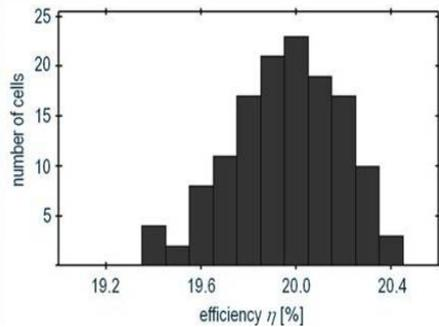
**Figure 5:** Best R&D cell run consisting of around 130 cells with a median cell efficiency of 20%, an open-circuit voltage of 646 mV, a short-circuit current density of 38.9 mA/cm<sup>2</sup> and a fill factor of 79.8% before light-induced degradation. Measurements were done at Q-Cells.
