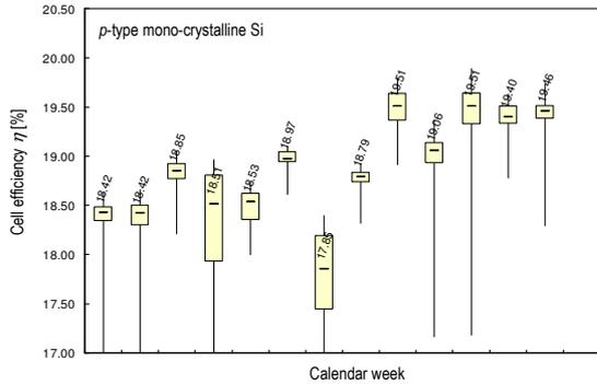
**Figure 4:** Recent results of the pilot series of mono-crystalline cells based on the Q.ANTUM cell technology at Q-Cells for different calendar weeks.
