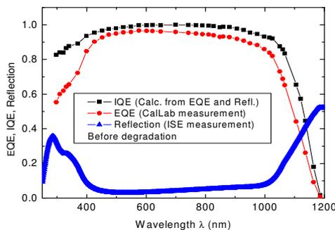
**Figure 3:** Results of the best cell of the joint experiment (group 3). External quantum efficiency (EQE) measured at Fraunhofer ISE CaLab, reflection characteristics measured at Fraunhofer ISE PV-TEC lab. Internal quantum efficiency (IQE) calculated from EQE and reflection.
