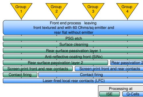
**Figure 2:** Process flow of 4 investigated groups. Laboratories in which the processes were performed are indicated.
