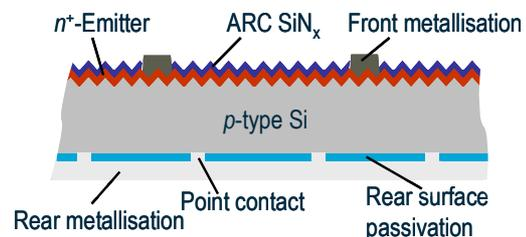
**Figure 1:** Schematic cross section of the Q.ANTUM cell.
