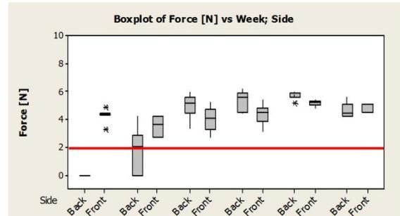
**Figure 6:** Soldering and adhesion tests of the front- and rear-side busbars. Due to optimisation of the metallization concept peel forces above 2 Newton are reached over several weeks.
