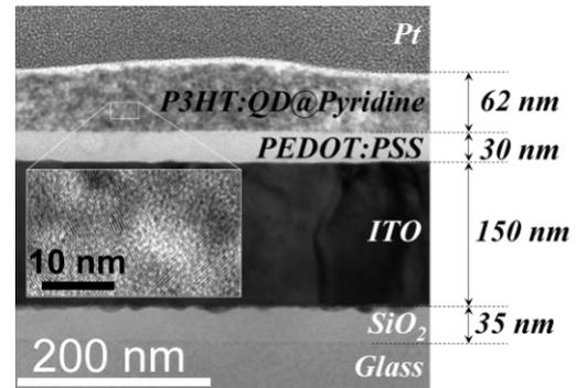
**Figure 3:** TEM image of the layer stack with a photoactive layer of P3HT blended with pyridine-capped QD ( $m=1:9$ ). The blend film shows a bright, polymer rich region at the interface to the metal back contact.
