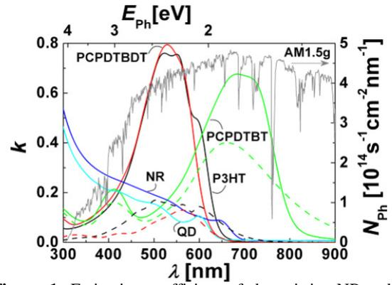
**Figure 1:** Extinction coefficient of the pristine NP and polymer films with layer thickness of approximately 90 nm and 70 nm, respectively. The polymers show uniaxial anisotropic behaviour with stronger extinction in the plane parallel to the surface (solid) as compared to the perpendicular direction (dashed). Isotropic OC were found for the NP-films.
