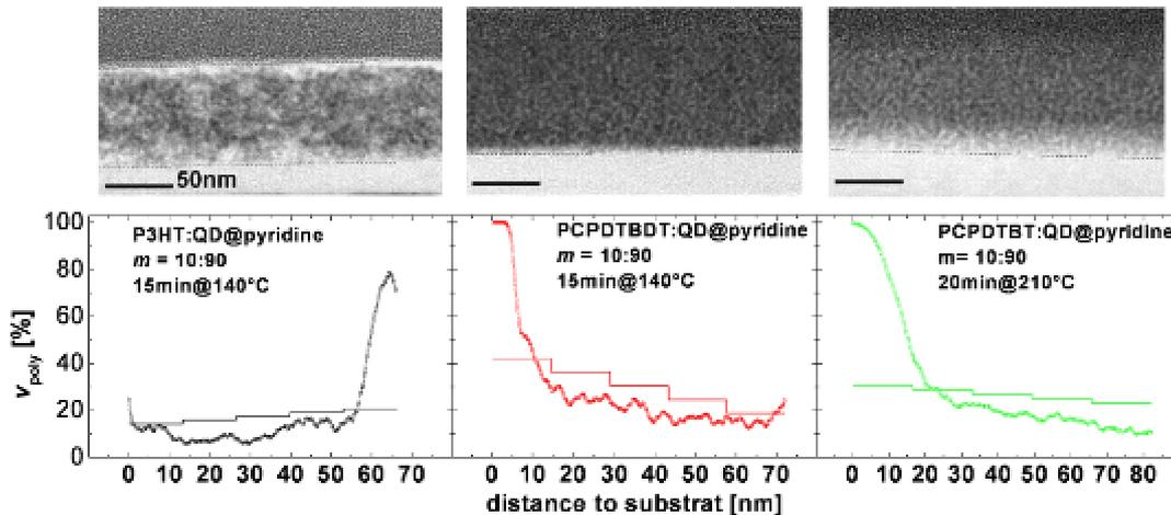
**Figure 4:** bottom: TEM- (circles) and EMA-gradient (lines) of the polymer:NP composition along the layer thickness. The TEM-gradient is a mean result of 8 (P3HT), 4 (PCPDTBDT) and 6 (PCPDTBT) images. top: representative TEM images of the blend films. The gradient was analysed in the area between the dotted lines.
