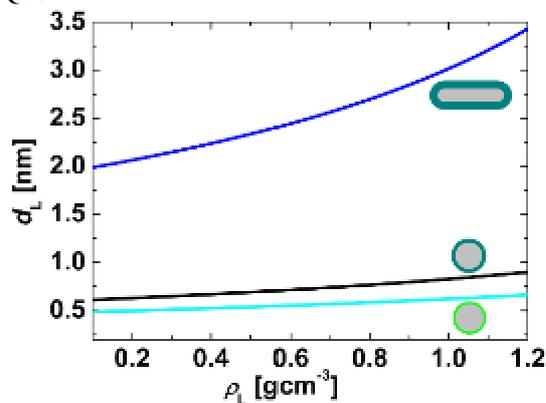
**Figure 6:** Ligand layer thickness as a function of its mass density. The plots result from the slope of the corresponding  $v(m)$ -trends and a geometrical representation of the particles in the blend with P3HT.
