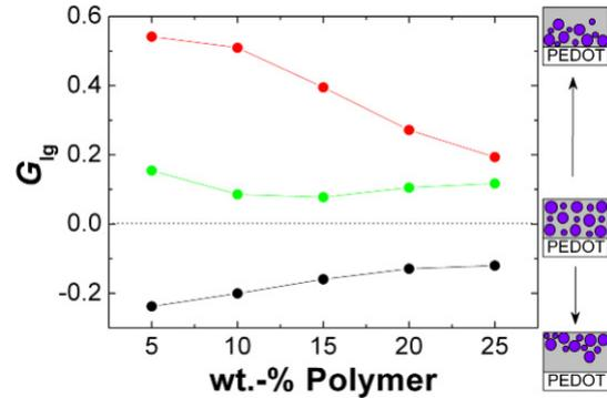
**Figure 2:** Logarithmic gradient of the polymer/QD volume composition for P3HT (black), PCPDTBDT (red) and PCPDTBT (green) blended with pyridine-capped QD. On the right a schematic representation of the gradient is shown (gray=QD, purple=polymer).
