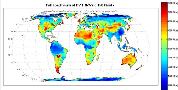
**Fig. 1:** Hybrid PV-Wind power plants characterized by their full load hours (FLh) projected for the year 2020. Assumed hybrid PV-Wind sub plants are 1-axis horizontal north-south continuous tracking PV power plants and wind power plants with a hub height of 150 m. The underlying resource data are provided by NASA SSE 6.0 [4] but further reprocessed [1].
