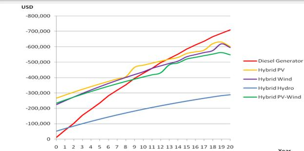
**Fig. 6:** Total cost of hybrid renewable mini-grid alternatives for an Ecuadorian village. In the long-term the diesel generator is typically the most expensive option, however the least cost option in the beginning. Micro-hydro would be the most cost competitive solution, if the hydro resource were available. In case of good solar and good wind resource availability, the hybrid PV-Wind mini-grid is typically the financial optimum.
