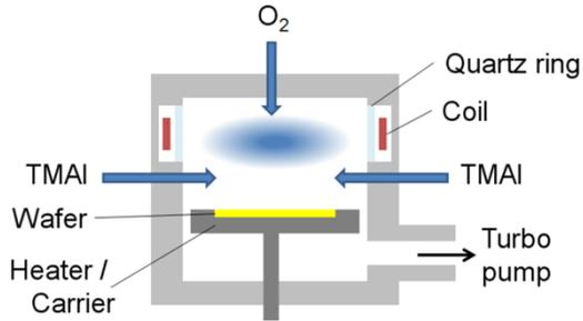
**Figure 1:** Schematic drawing of the laboratory-type ICP  $\text{AlO}_x$  deposition chamber. The plasma is inductively excited with a coil outside the vacuum chamber using TMAI and  $\text{O}_2$  as process gases. The wafer is transported on a carrier and heated during deposition.
