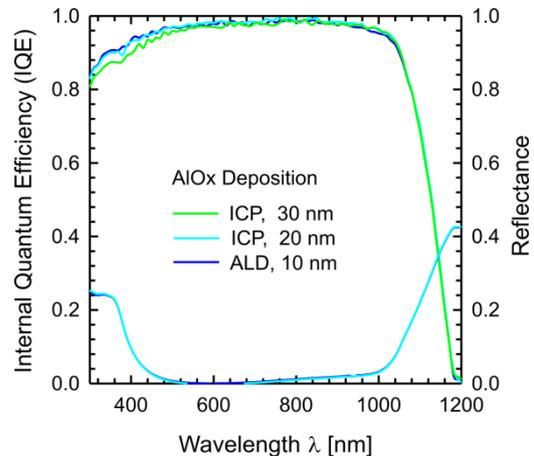
**Figure 5:** Internal quantum efficiency (IQE) and reflectance of the PERC solar cells of table 1. By analytical modeling we obtain  $S_{rear}$  values of 60 – 120  $\text{cm}/\text{s}$  and an  $R_b$  of 90 – 92% showing the excellent electrical and optical parameters of the ICP  $\text{AlO}_x/\text{SiN}_y$  passivation stacks.
