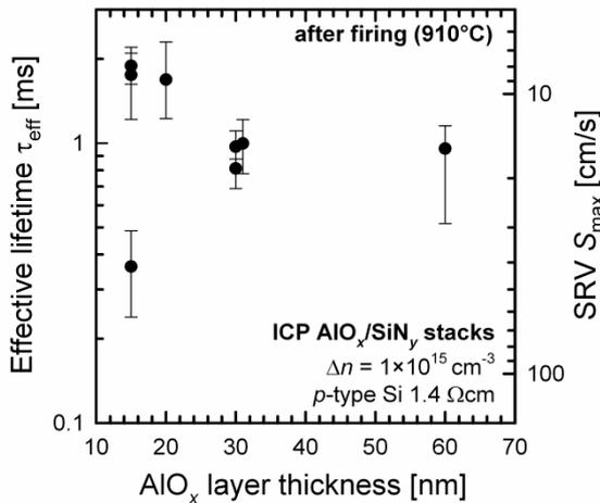
**Figure 2:** Effective carrier lifetime and corresponding surface recombination velocity measured on 1.4  $\Omega\text{cm}$  float zone (FZ) wafers in dependence of the ICP  $\text{AlO}_x$  layer thickness showing lifetimes of up to 2 ms and surface recombination velocities below 10 cm/s for ICP  $\text{AlO}_x$  layers covered with a  $\mu$ W-PECVD  $\text{SiN}_y$  layer (SiNA, Roth und Rau) after firing.
