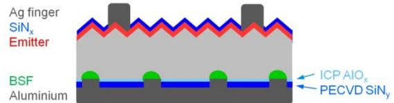
**Figure 3:** Schematic drawing of the PERC solar cells processed at ISFH with screen-printed front and rear contacts applying a ICP  $\text{AlO}_x/\text{SiN}_y$  rear passivation stack.
