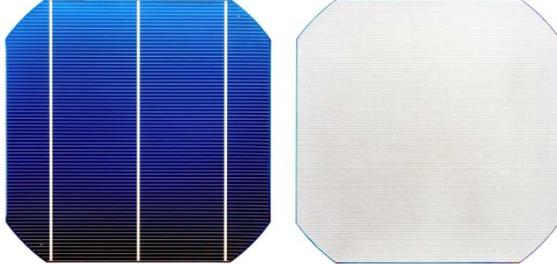
**Figure 4:** Photographs of the front and rear side of a PERC solar cell with 20.1% conversion efficiency. Whereas the front side is very similar to industry-standard screen-printed solar cells, the rear side shows the ICP  $\text{AlO}_x/\text{SiN}_y$  passivation layer and the local line contacts.
