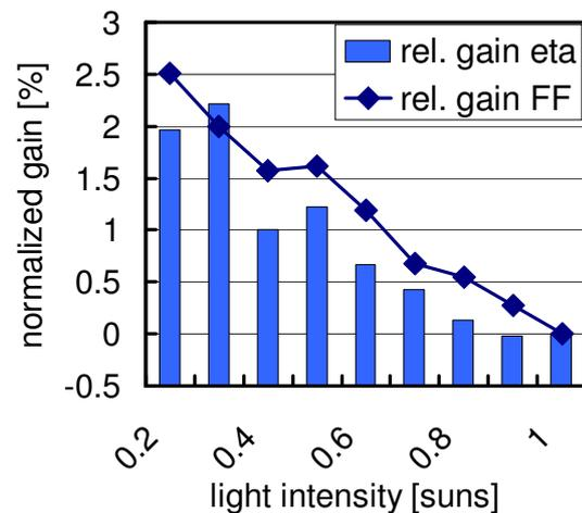
FIG. 7. Weak light behaviour of Q.ANTUM modules, shown is the normalized relative gain compared to Al-BSF Modules of the fill factor and the efficiency as a function of the illumination intensity.
