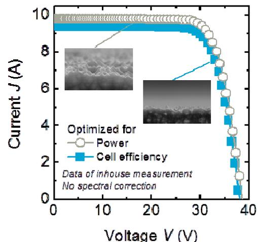
FIG. 4.  $I$ - $V$  characteristics of our new world record efficiency (multi) and power (mono-cast) module.
