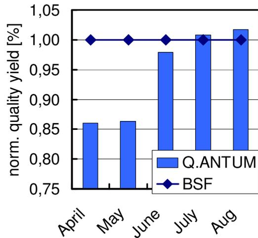
FIG. 6. Evolution of the quality yield of the Q.ANTUM production normalized to the BSF reference process. Starting around 15% below the BSF reference, now similar values are reached.
