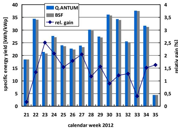
FIG. 8. Specific weekly energy yield of Q.ANTUM and Al-BSF PV system installed near Thalheim for the last half year.
