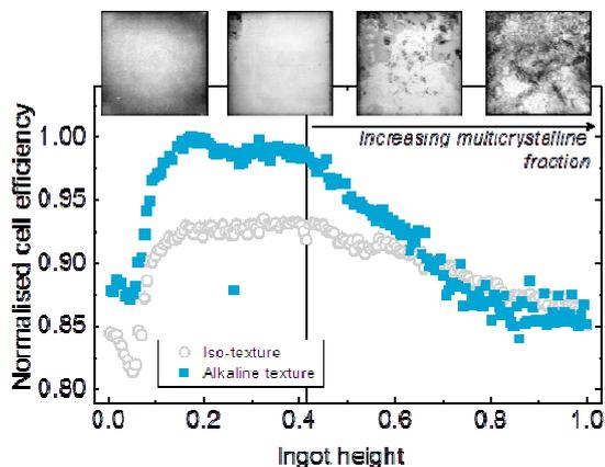
Fig. 2: Normalized efficiencies of multi-cast and mono-cast cells with either isotropic or alkaline textured front side.
