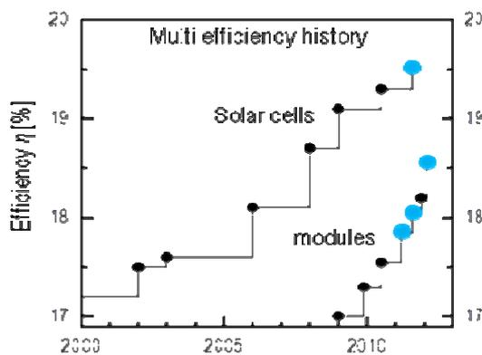
FIG. 1. Reported record solar cell and module efficiency history on multi-crystalline Si [2].
