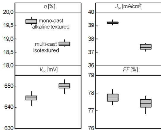
FIG. 3.  $I$ - $V$  characteristics of Q.ANTUM solar cells used for our new world record modules. The multi-cast cells feature an isotextured surface whereas the mono-cast cells are alkaline textured.
