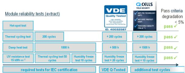
FIG. 9. Performed module reliability test (extract) with Q.ANTUM modules.
