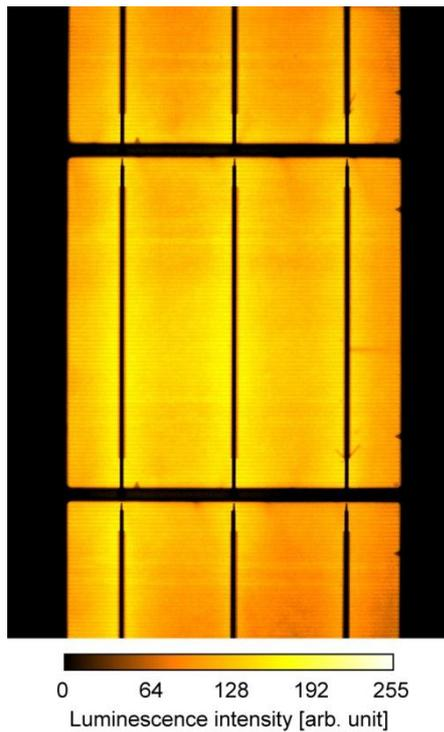
**Figure 6:** Electroluminescence image of a representative mono-crystalline cell in a test specimen after lamination (displayed in false color representation).
