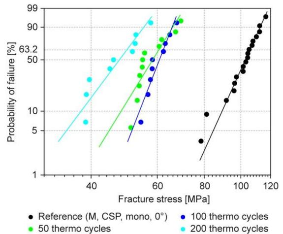
**Figure 7:** Weibull plot of crack occurrences in standard test specimens including mono crystalline cells (M, CSP, mono, 0°, TCT) after different number of thermo cycles.
