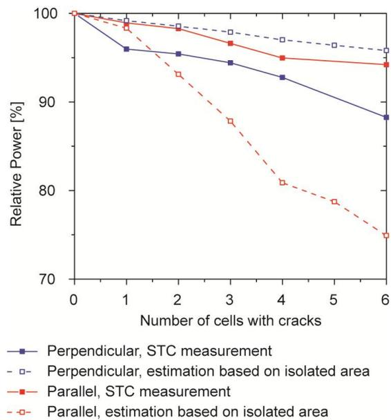
**Figure 5:** Relative power output of test specimens with cell cracks (power corresponds to total power of the six cells in the middle of the test specimen).
