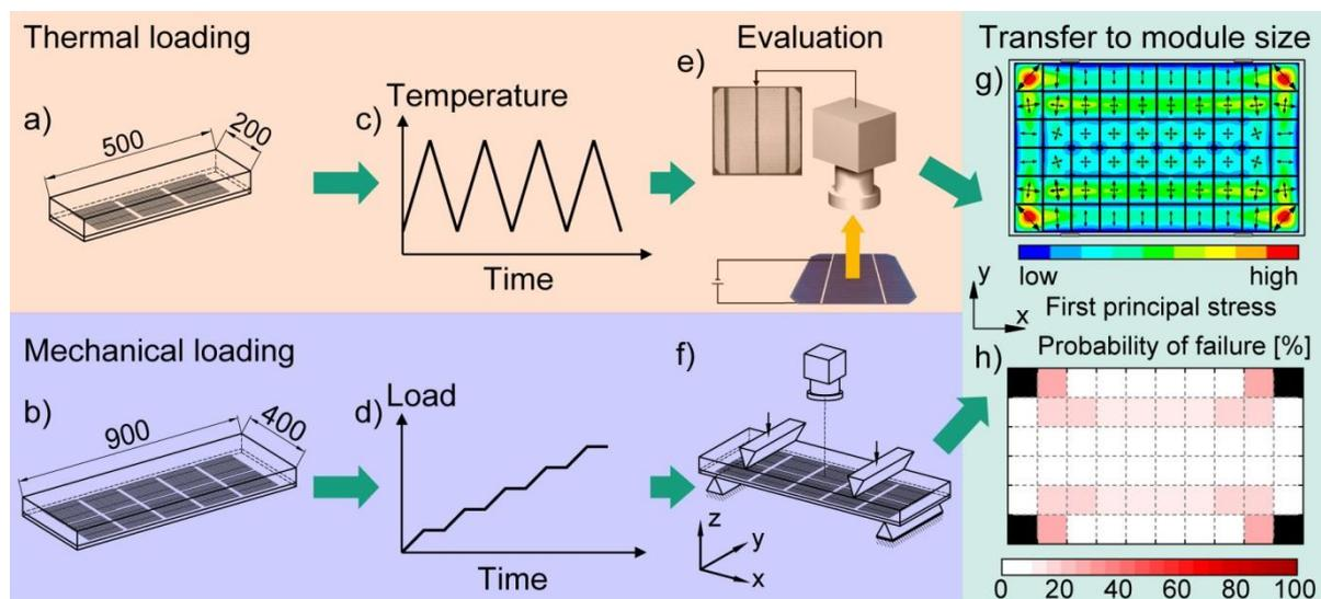
**Figure 1:** Experimental approach for separate investigation of thermal and mechanical loading.
