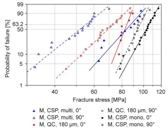
**Figure 3:** Weibull plot of the crack occurrences in standard test specimens including multi-crystalline and mono-crystalline cells with a thickness of 180  $\mu\text{m}$ .
