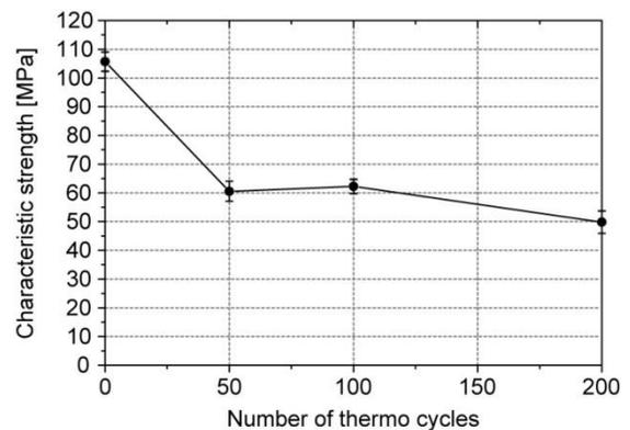
**Figure 8:** Characteristic strength of mono crystalline cells in standard test specimens plotted for different number of thermo cycles.
