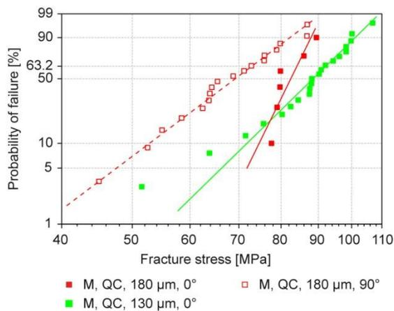
**Figure 4:** Weibull plot of crack occurrences in standard test specimens including multi crystalline cells with variable thickness.
