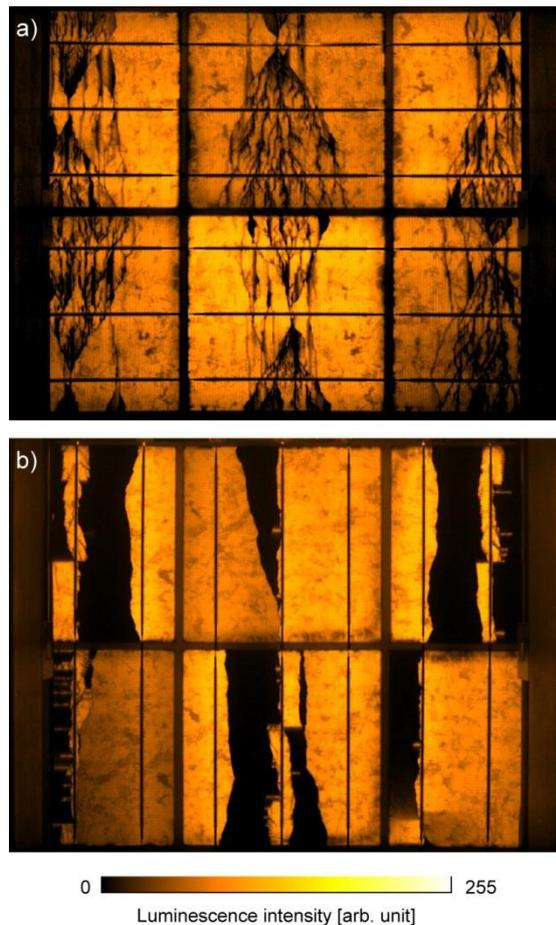
**Figure 2:** Electroluminescence image of the middle cells of test specimens including multi-crystalline cells during 4-point bending; (a) M, QC, 180  $\mu\text{m}$ , 0°, perpendicular to the busbars; (b) M, QC, 180  $\mu\text{m}$ , 90°, parallel to the busbars (displayed in false color representation).
