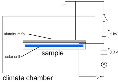
**Figure 1:** Schematic of the experimental setup for PIS and regeneration from PIS.
