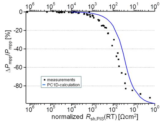
**Figure 3:** Measured relative loss of  $P_{mpp}$  versus  $R_{sh,PIS}(RT)$  normalized to the cell area for single-cell modules. The blue line represents model calculations assuming ohmic shunting only.
