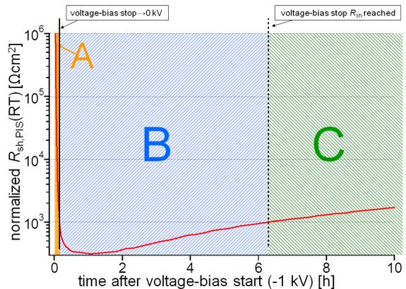
**Figure 6:**  $R_{\text{sh,PIS}}$ -measurement of a single-cell module during and after PIS at  $90^\circ\text{C}$ . The  $R_{\text{sh,PIS}}$ -behavior can be separated into 3 distinct phases: shunting (A), transition phase (B) and regeneration (C).
