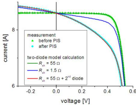
**Figure 4:** Comparison of  $I$ - $V$  curves before and after PIS with simulated curves assuming ohmic shunt behavior only (green and blue line) or with nonlinear shunting (red line).
