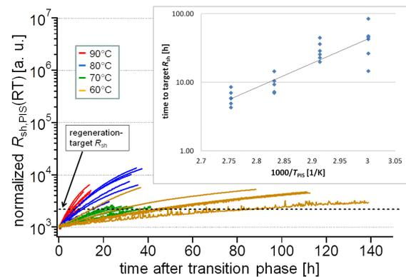
**Figure 9:**  $R_{sh,PIS}$ -measurement of single-cell modules at different temperatures and zero voltage bias after PIS. The regeneration target value is depicted by a dashed horizontal line. In the inset an Arrhenius plot of the time to reach the regeneration target value is shown.
