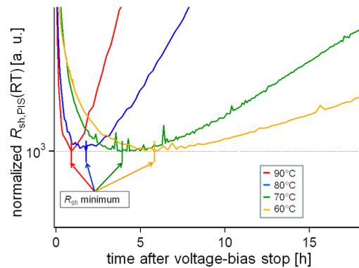
**Figure 8:**  $R_{sh,PIS}$ -measurement of single-cell modules directly after PIS at different temperatures. The  $R_{sh,PIS}$ -measurements are normalized to the curve minima which are depicted by vertical lines.
