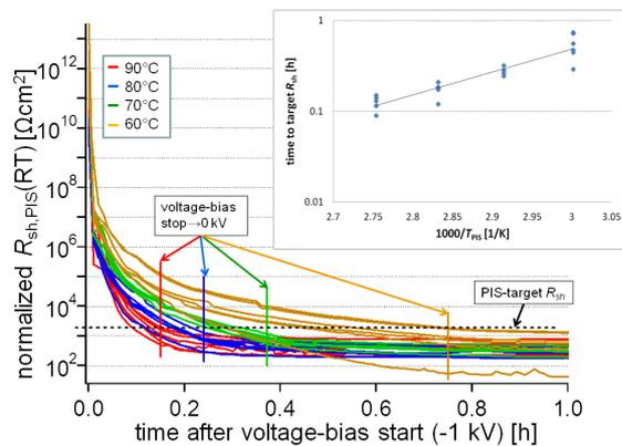
**Figure 7:**  $R_{sh,PIS}$ -measurement of single-cell modules during PIS at different temperatures. The voltage bias stop and the PIS target value are depicted by vertical and horizontal lines, respectively. In the inset an Arrhenius plot of the time to reach the PIS target value is shown.
