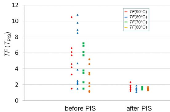
**Figure 2:**  $R_{sh}$  temperature factors ( $TF(T_{PIS})$ ) for single-cell modules before and after PIS at different temperatures.
