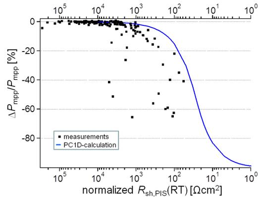
**Figure 5:** Measured relative loss of  $P_{\text{mpp}}$  versus  $R_{\text{sh,PIS}}(\text{RT})$  per cell normalized to the area of one cell for 60-cell modules. The blue line represents model calculations assuming ohmic shunting only.
