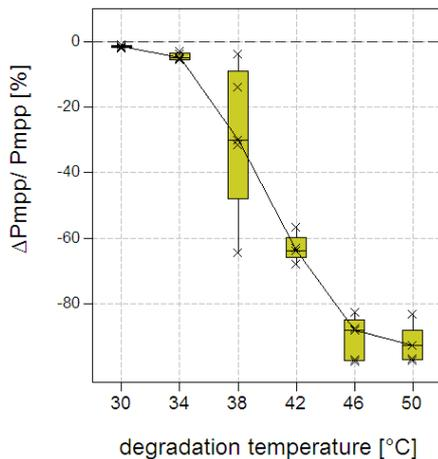
**Figure 5:** Effect of the temperature to the intensity of degradation. Test series with medium PID-vulnerable cells (v3). Degradation time 23 h; applied bias voltage 13 kV.
