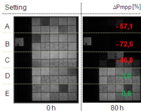
**Figure 7:** EL-images and performance measurement of the crosscheck PID-module (ten cells per setting = one string). Test conditions: -1 kV, aluminum foil on front, degradation temperature 49°C.
