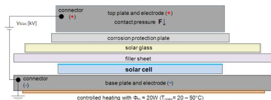
**Figure 1:** Principle schematic of the press-stack construction used for the PID-test for un laminated solar cells
