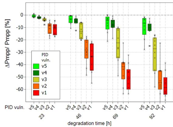
**Figure 3:** Effect of specific PID-vulnerable samples to the result of degradation. Test series with five nominal different PID-vulnerabilities. Highest vulnerability is v1, lowest is v5. Applied voltage is 13 kV; degradation temperature is 34°C.
