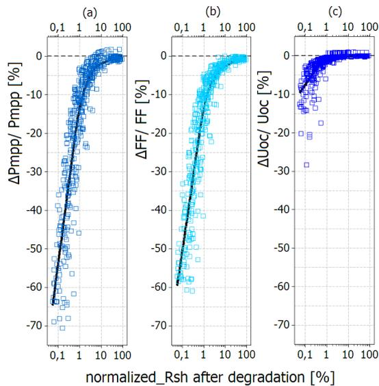
**Figure 2:** (a) Measured  $\Delta P_{mpp} / P_{mpp} [\%]$  versus  $R_{sh} [\%]$  after degradation.  $R_{sh}$  is normalized to the initial values before degradation. Analogous (b) measured  $\Delta FF / FF [\%]$  and (c) measured  $\Delta U_{oc} / U_{oc} [\%]$ . The data basis consists of 475 individual measurements of unlaminated p-type solar cells with different PID-vulnerabilities after application of various degradation parameters. The black lines are smoothing functions.
