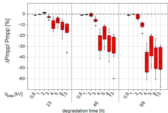
**Figure 4:** Effect of the applied bias voltage to the result of degradation. Test series with PID-vulnerable cells (v1). Degradation temperature is 34°C.
