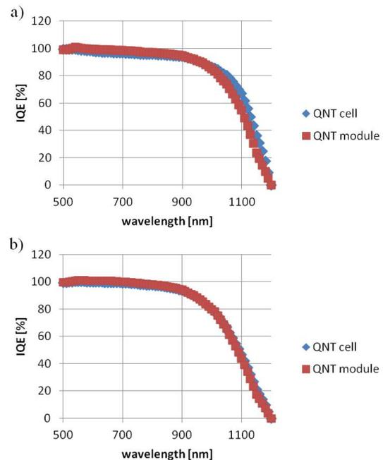
**Figure 5:** Quantum efficiency curves of Q.ANTUM cells before and after encapsulation with a) wrong and b) optimized module built parameters.
