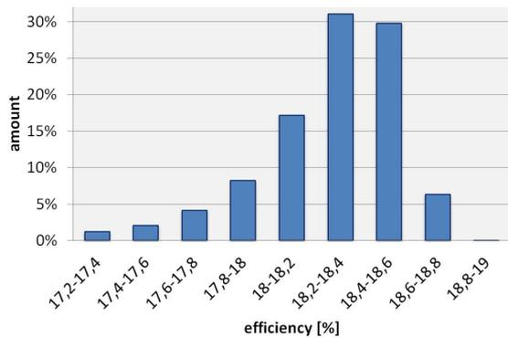
**Figure 3:** Distribution of cell efficiencies of a typical Q.ANTUM cell production run.
