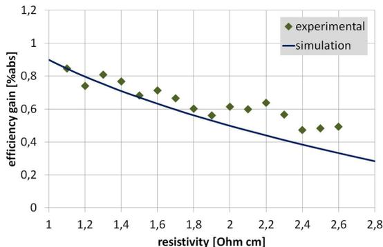
**Figure 4:** Experimental and simulated efficiency gain of Q.ANTUM relative to Al-BSF cells on sorted material.
