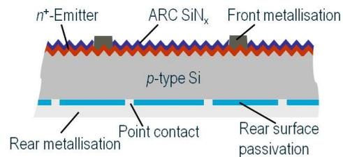
**Figure 1:** Schematic cross section of the Q.ANTUM solar cell design.
