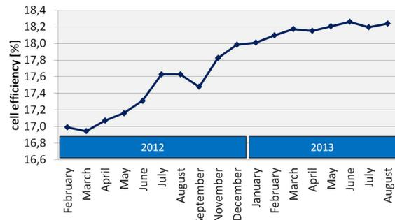
**Figure 2:** Average efficiency per month of the Q.ANTUM pilot line production in 2012/2013.
