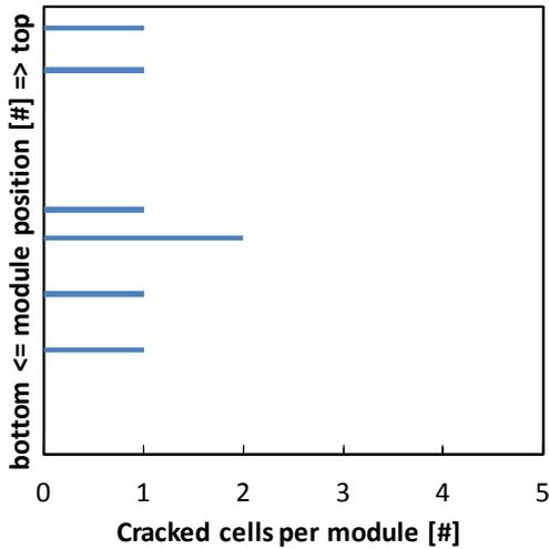
Fig. 4: Some PV modules in the transport stack show one or two cell cracks per PV module after the transport. This statistic belongs to the same transport being evaluated in Fig. 3 a) and c).
