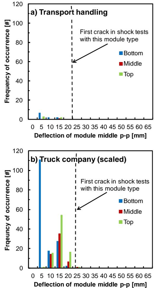
Fig. 9: Deflection occurrence for a truck company transport calculated by applying the mean transfer function of Fig. 5 with Eq. (2) to the base acceleration data used to generate Fig. 3 c). For that module type the dashed line indicates the module deflection where the first cell cracking occurs in the shock tests, compare Fig. 8.
