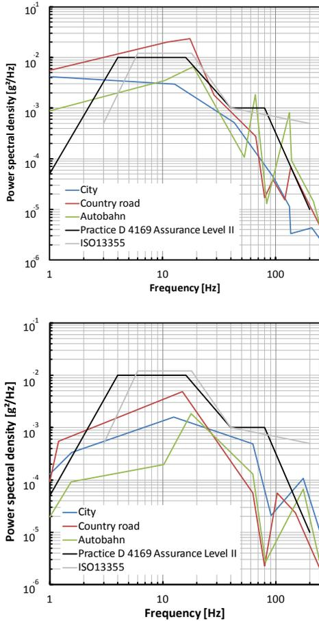
Fig. 10: Measured reduced PSDs of a transport stack for sunny side down stacked PV modules. The PSD is measured in the corners of PV modules. a): upper PV module in the stack, b): bottom PV module in the stack. The reduced PSDs are created according to the standard DIN EN 15433-5 Feb2008. The grey and black PSD-curves are similar standard spectra.
