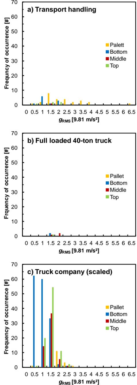
Fig. 3: Measured shock occurrence for a) transport handling, b) transport in full loaded 40-ton truck and c) transport with a truck company driving the same distance. Pallet, bottom, middle and upper indicate the measurement at the module positions at the pallet and in the bottom, middle and upper part of packaging unit.
