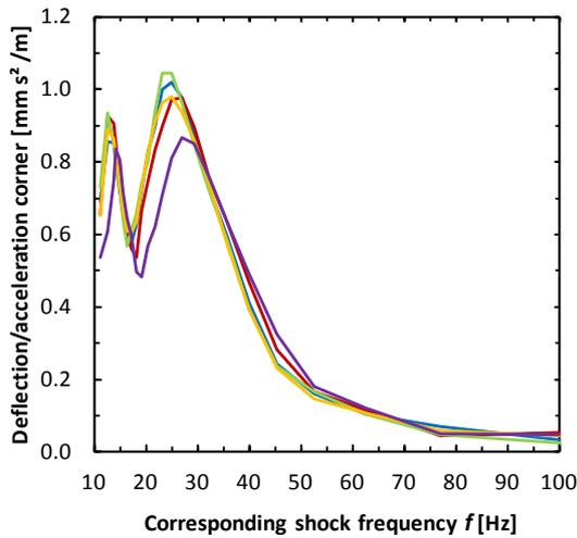
Fig. 7: Normalized deflection functions as function of the corresponding shock frequency for 5 different module types.
