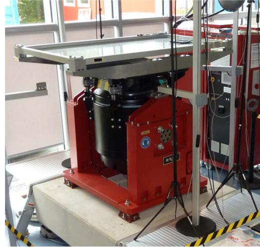
Fig. 2: Photograph of the shaker setup.
