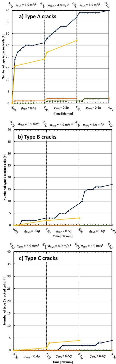
Fig. 12: The cumulative cell cracking as function of the time of the module under vibration for 4 exemplary PV module types. The mean acceleration  $g_{RMS}$  is increased after 3h and 6 h of test. Occurrence of cells showing crack type A is shown in fig a), type B in b) and type C in c).
