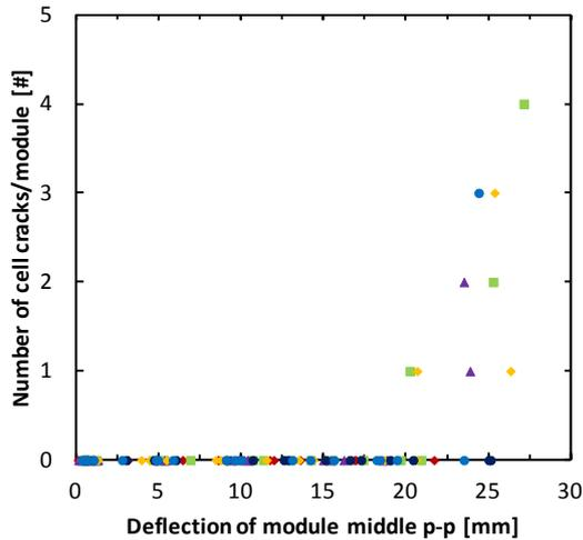
Fig. 8: Correlation of the maximum deflection of the module to the number of generated cell cracks. Different points represent different PV module types, shocked for several amplitudes  $a_{max}$  and corresponding shock frequencies  $f$  resulting in a certain deflection.
