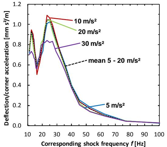
Fig. 6: The functions given in Fig. 5 scaled by the corresponding shock amplitude  $a_{max}$  given as parameter in the graph. Up to  $a_{max} = 20 \text{ m/s}^2$  peak acceleration all functions scale linear with the shock amplitude. For  $30 \text{ m/s}^2$  the functions still scale linear except for the peak regions.
