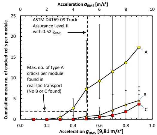
Fig. 11: The graph shows the cumulative mean number of solar cells with new cracks of type A, B and C after a 15 min noise test using the ASTM D4169-09 Truck PSD spectrum. The RMS acceleration amplitude  $g_{RMS}$  of the PSD is varied in this experiment. The bars show the maximum variance of the set of tested PV modules.
