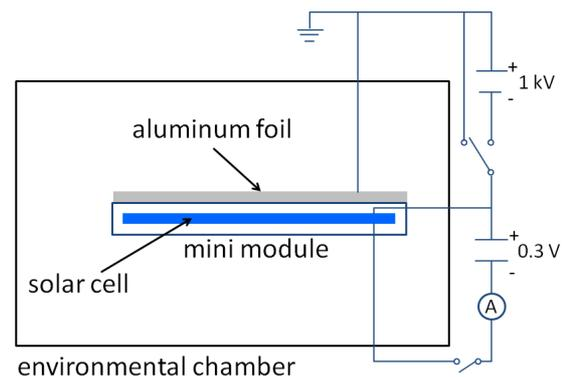
**Figure 1:** Schematic of laboratory setup
