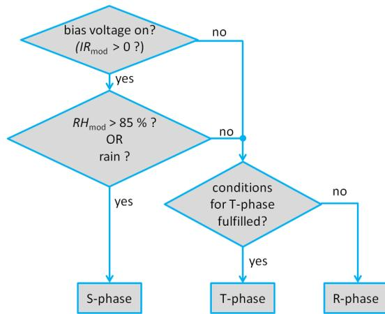
**Figure 5:** Illustration of phase-assignment process for every time step of the simulation
