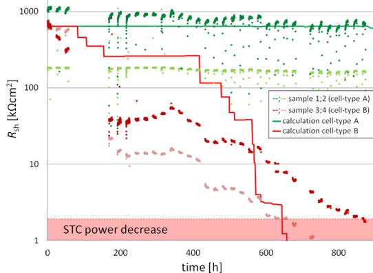
**Figure 8:** Night-time measurement of  $R_{sh}$  over time of fielded mini-modules (dashed lines) together with  $R_{sh}$  model calculations (solid lines).
