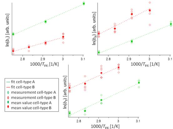
**Figure 7:** Arrhenius-plots of  $b_S$ ,  $b_T$  and  $b_R$  for mini modules with two different cell types. The measured data (open symbols), mean values (solid symbols) and Arrhenius fits (dashed lines) are shown.
