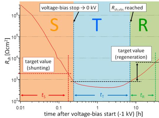
Figure 4:  $R_{sh}$  measurement over time of a mini-module during and after PID-s at a fixed temperature. The progression is divided into shunting (S)-, transition (T)- and regeneration (R)-phase
