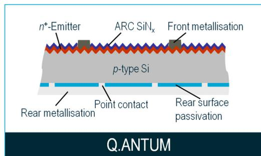
Fig. 6. Schematic cross section of a Q.ANTUM cell [6]. The Al-BSF at the rear side of a standard Al-BSF cell is replaced by a rear surface passivation layer with local point contacts.
