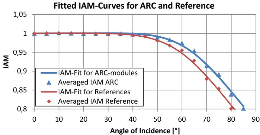
Fig. 3. The line plots are fitted IAM-curves as input for the energy yield simulation. The symbols show IAM value averages of two modules and over 5°.
