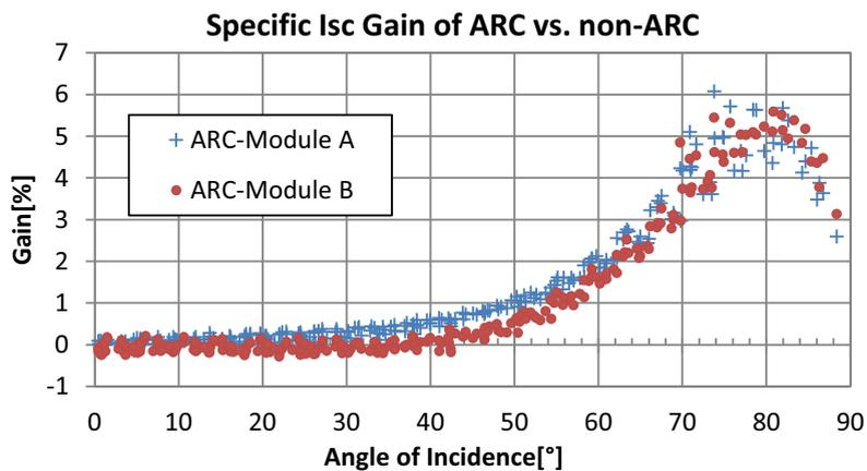
Fig. 2. Specific  $I_{sc}$  gain of two ARC-modules with respect to average of two non-ARC-modules (zero). Both ARC-modules show a rising gain for increasing incident angles larger  $45^\circ$  with a maximum of approximately 5% at an incident angle of  $80^\circ$ .
