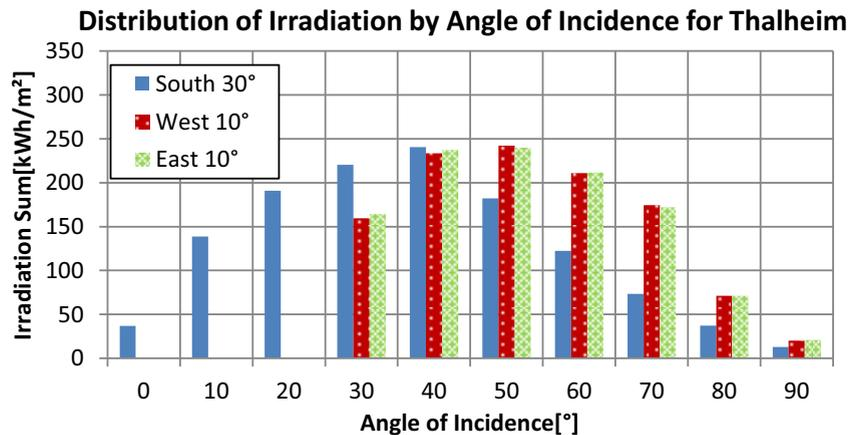
Fig. 4. Distribution of global irradiance for different system orientations and inclination angles by the angle of incidence. The presented values are calculated using the angle of incidence [4] and global and direct irradiation measurements. The diffuse component is assumed as isotropic.
