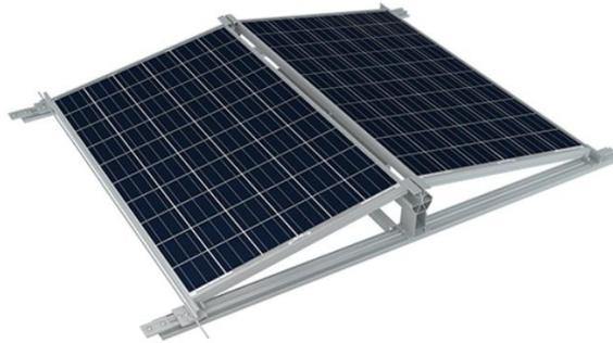
Fig. 5. The Hanwha Q CELLS flat roof solution Q.FLAT-G3 increases the roof space utilization to up to 82% - twice as much as an installation with  $30^\circ$  inclination. The modules are facing east and west with an inclination angle of  $10^\circ$  [8].
