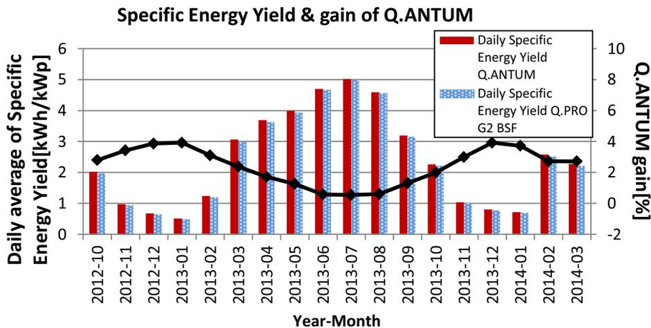
Fig. 8. Measured Specific Energy Yield gain of Q.ANTUM compared to Q.PRO-G2 (BSF). The Q.ANTUM system shows a gain of at least 0.5% and rises to up to 4% in the winter months.
