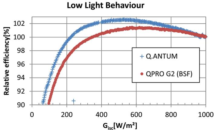
Fig. 7. Low light behavior of a module with Q.ANTUM cells (blue circles) and a module with Al-BSF cells (red dots). A significant improvement in low light behavior can be observed for all irradiances below 1000W/m<sup>2</sup>. For an irradiation of 200 W/m<sup>2</sup>, a difference of 2.5% can be observed.
