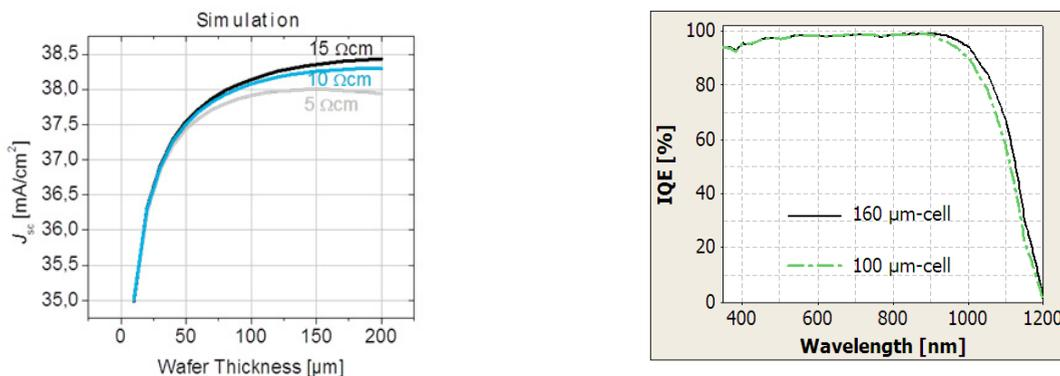
Fig. 2. Left: Insufficient light trapping causes steep decline in  $J_{sc}$  for wafer thicknesses < 100  $\mu$ m. Right: 100  $\mu$ m thin cells show an IQE loss for long wavelengths compared to 160  $\mu$ m cells corresponding to the  $J_{sc}$  loss.
