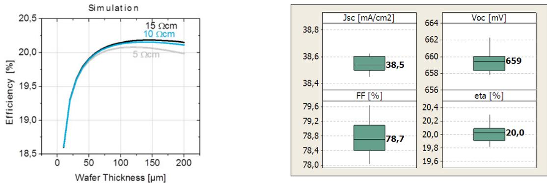
Fig. 4. Left: Simulated cell efficiency as a function of wafer thickness for different base resistivities. Wafer thicknesses between 100 and 200 μm result in highest efficiencies. Right: Measured cell parameters of 100 μm-thin cells: median cell efficiency of 20 % is shown.
