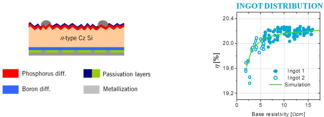
Fig. 1. Left: Cross section of the double-side contacted rear junction solar cell investigated within this article. Right: The cell results along an ingot distribution are fitted to obtain input parameters for PC1D.
