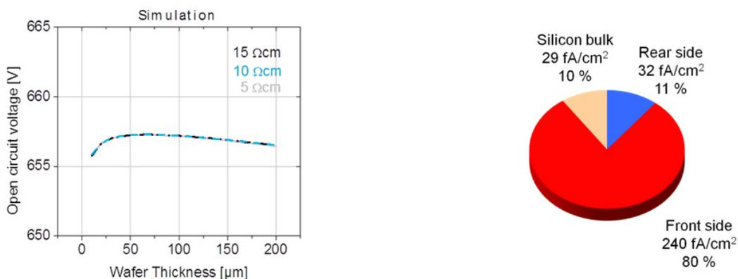
Fig. 3.  $V_{oc}$  increases only slightly for thinner wafers (left) due to small  $J_0$  contribution of bulk (right).
