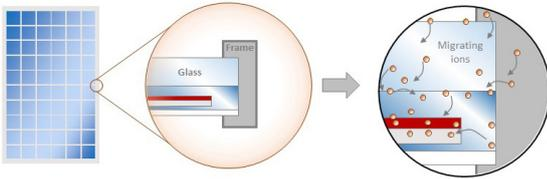
Figure 5: Migrating sodium ions in PV module, the force behind PID
