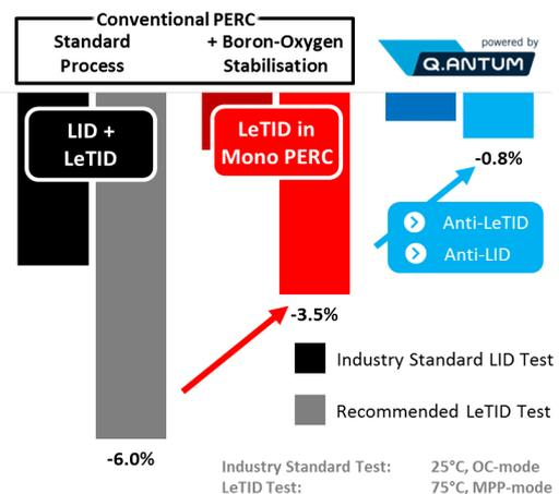
Figure 4: Observable degradation from industry standard LID test and LeTID testing for differently processed PERC modules.
