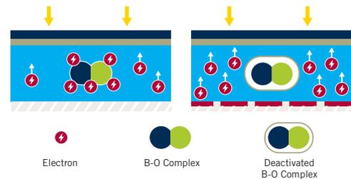
Figure 3: Boron-Oxygen complex in standard cell and Deactivated Boron-Oxygen complex in Q.ANTUM cell
