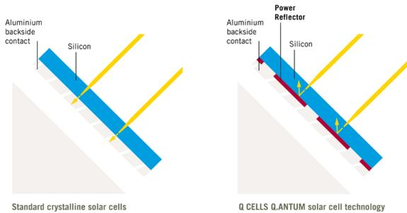
Figure 1: Additional "Power reflector" in Q.ANTUM solar cells
